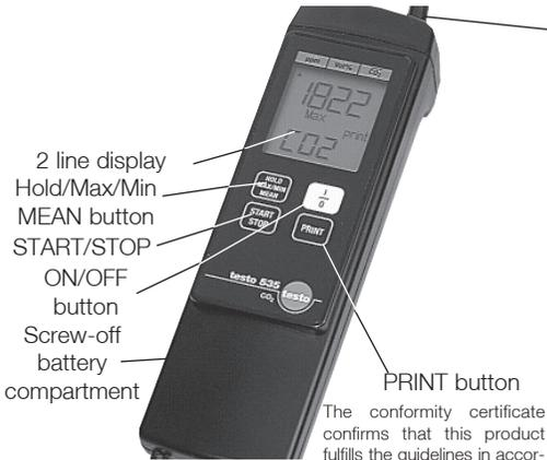
Mains connection (mains unit no. 0554.0088) recommended for long-term measuring.
